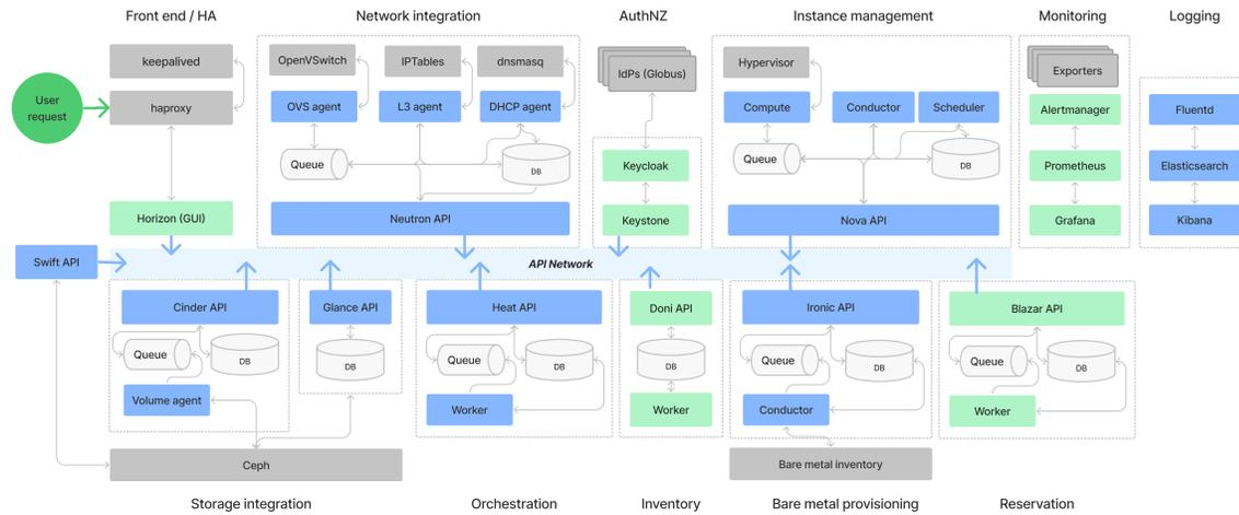
Fig. 1. CHI-in-a-Box services and relationships. The items in green denote additional services contributed by Chameleon, or services with significant capabilities not available upstream.
